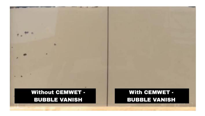
With **CEMWET – BUBBLE VANISH**, the surface of secondary concrete becomes Bubble Free.
